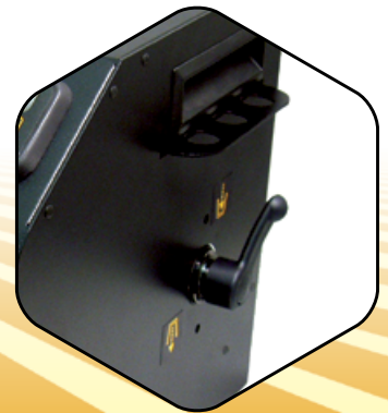
Release Lever to Dump Grain
