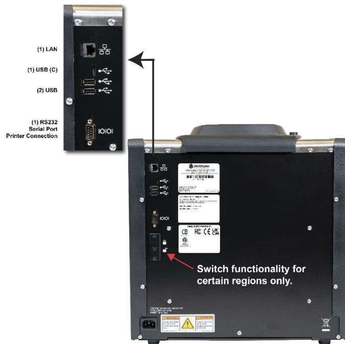
Figure 2 External Communication Connections (Back of Unit)
