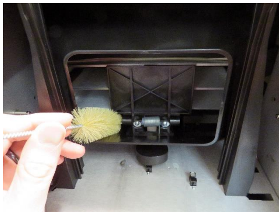
Figure 13 Clean Under Trap Door
