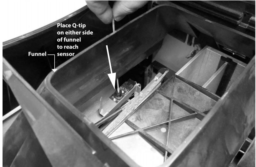
6. Allow the temperature sensor to dry for 90 seconds then gently clean with the dry end of the cotton swab.
