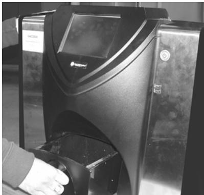
4. Using the supplied brush, manually remove any loose or stuck grain or dust from the measuring cell.
