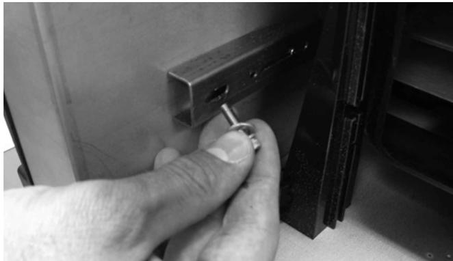
7. Press down on the bracket to release.
