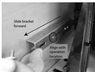
5. Slide bracket forward and align with operation location.
