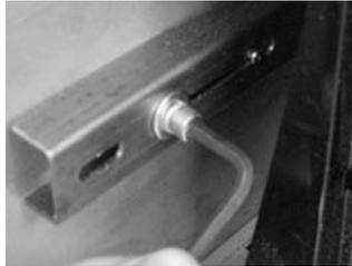
6. Insert hex bolt into operating location hole and tighten using the Allen wrench.
