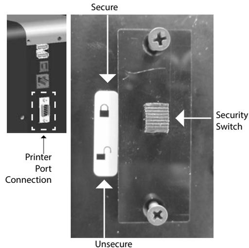
**NOTE:** When the switch is toggled from secure to unsecure, an event is logged into memory for traceability.
