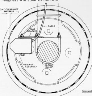
5. Refer to the above illustration and install the U-bolt clamp on the spindle between the
