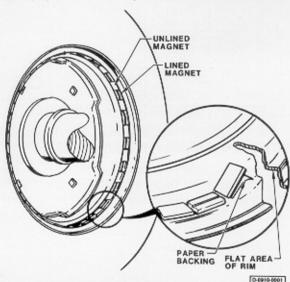
3. Refer to the above illustration and place the magnets around the flat area of the rim. Do not remove the paper backing from the magnets at this time. The magnets must alternate (lined then unlined) around the circumference of the rim. If two like magnets (lined or unlined) end up together or close enough that another magnet will not fit when the rim is full, then one magnet must be added to or deleted from the magnet ring.
