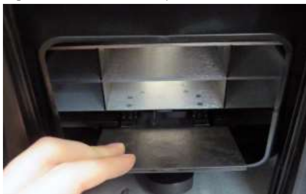
Figure 10 Pull Down on Trap Door
