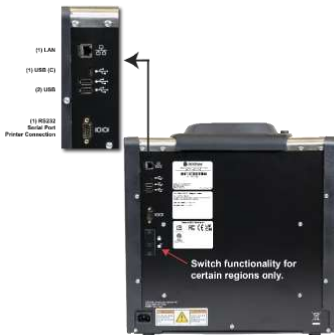
Figure 2 External Communication Connections (Back of Unit)
