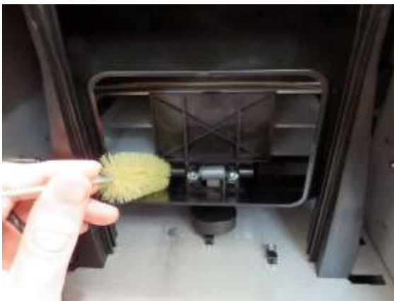
Figure 12 Clean Under Trap Door
