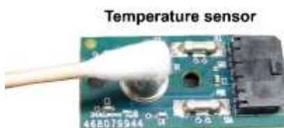
Figure 16 Magnified View of Proper Cleaning with Cotton Swab
