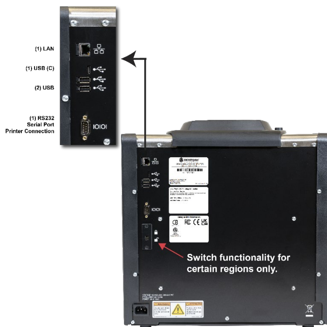
Figure 2 External Communication Connections (Back of Unit)
