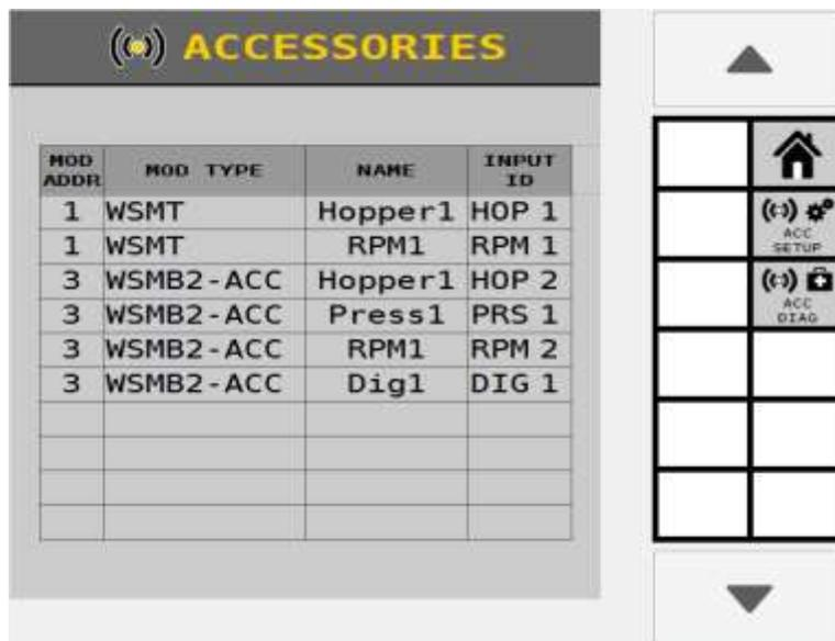
The Accessory Setup screen allows accessory sensors to be configured for each supported accessory module. Pressing the **NEXT MODULE** softkey navigates through each supported accessory module to setup sensors for the selected module.
