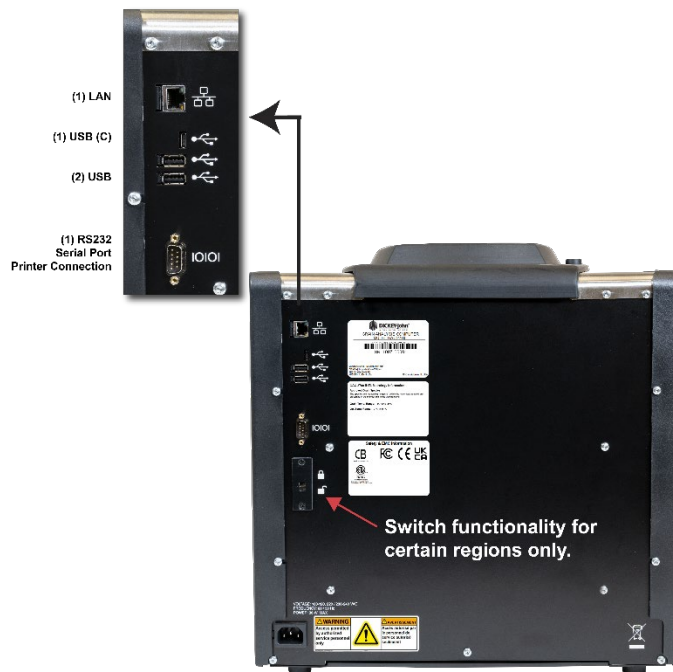
Figure 2 External Communication Connections (Back of Unit)
