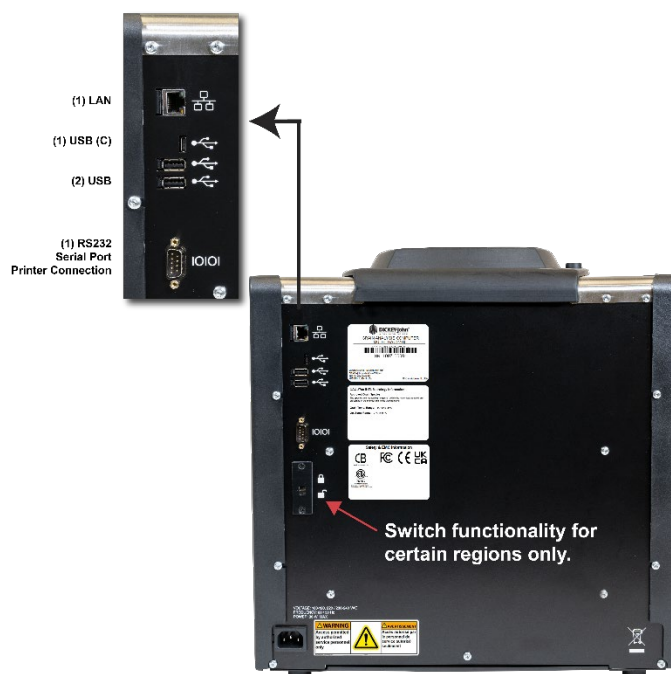
Figure 2 External Communication Connections (Back of Unit)
